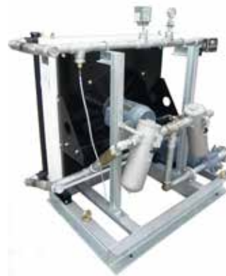
Oil cooling package fitted with ST75 model heat exchanger, Haight pump and duplex filter. Sensors for oil flow, oil temperature, oil pressure and filter condition. Thermostatic control of fan motor.
